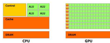
Figure 1-2. The GPU Devotes More Transistors to Data Processing
