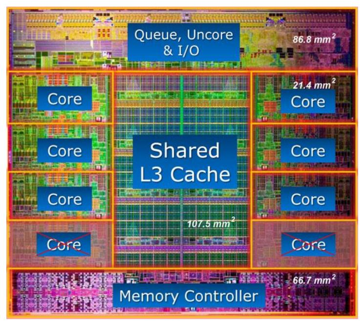
Intel Core i7 3960X (Codename Sandy Bridge-E) – 2.27B transistors, Total Size 435mm<sup>2</sup> Source: www.lostcircuits.com
