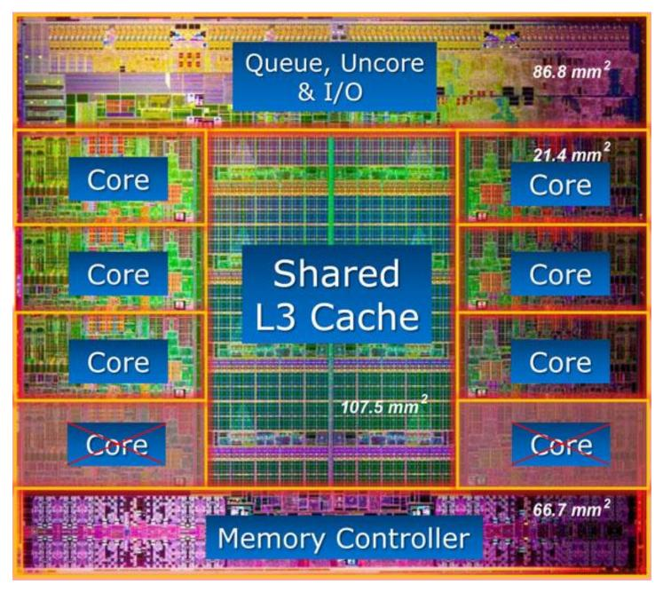
Intel Core i7 3960X – 15MB L3 (25% of die). 4-channel Memory Controller, 51.2GB/s total Source: www.lostcircuits.com
